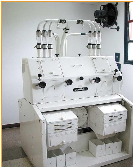
**Figura 16- Molino experimental Buhler 202D**
